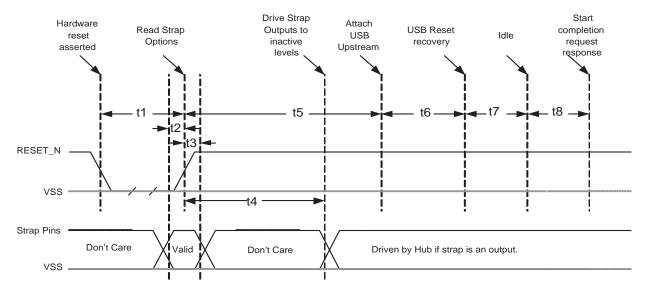
Figure 4.3 Reset\_N Timing for Default/Strap Option Mode
